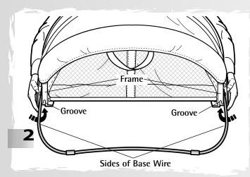
Lift the product up slightly so that each side of the base wire "snaps" into the groove in each frame. Make sure you hear a "snap".
